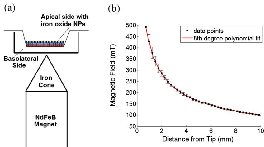
**Fig. 1** **a** Schematic of experimental system to generate and apply focused high magnetic field gradient due to a permanent neodymium (NdFeB) magnet with an iron cone pole piece to primary normal human tracheobronchial epithelial (NHTE) cells. NHTE cells are depicted in red and mucus layer is depicted in blue. The apical side mimics the airway lumen and the basolateral side mimics the airway
