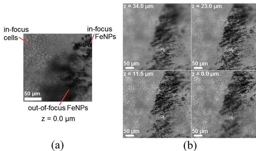
**Fig. 5** Bright field image of primary human airway epithelial cells (*gray*) and PVP coated 20–30-nm  $\text{Fe}_3\text{O}_4$  magnetic nanoparticle (FeNP) aggregates (*black*). The sample was exposed to a magnetic field gradient of  $60 \pm 3$  T/m for 1 h. **a** Some FeNPs (in-focus FeNPs) successfully penetrated the 100- $\mu\text{m}$  thick mucus and reached the cell
