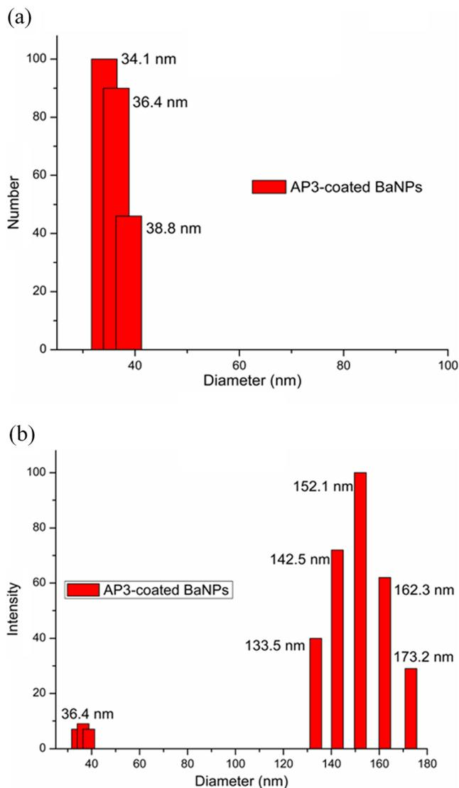
**Fig. 2** **a** Number-weighted size distribution of milled AP3-BaNPs. The majority of NPs were 34.1 nm in diameter. **b** Intensity-weighted size distribution of milled AP3-BaNPs. A small portion (<1 % by number) of NPs ranged from 133.5- to 173.2-nm diameter
